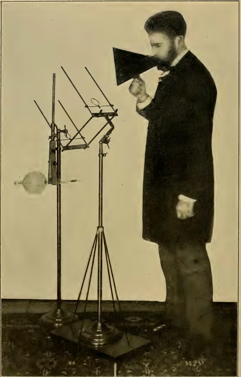
PLATE 60.—This instruction plate shows Author's Frame and Localizer with a pair of rings substituted for rod markers to define a small field for examination. Also shows how frame can be tilted to any angle to engage axis of rays. Press the part to be examined close against ring on front and it will be in path of vertical rays.
